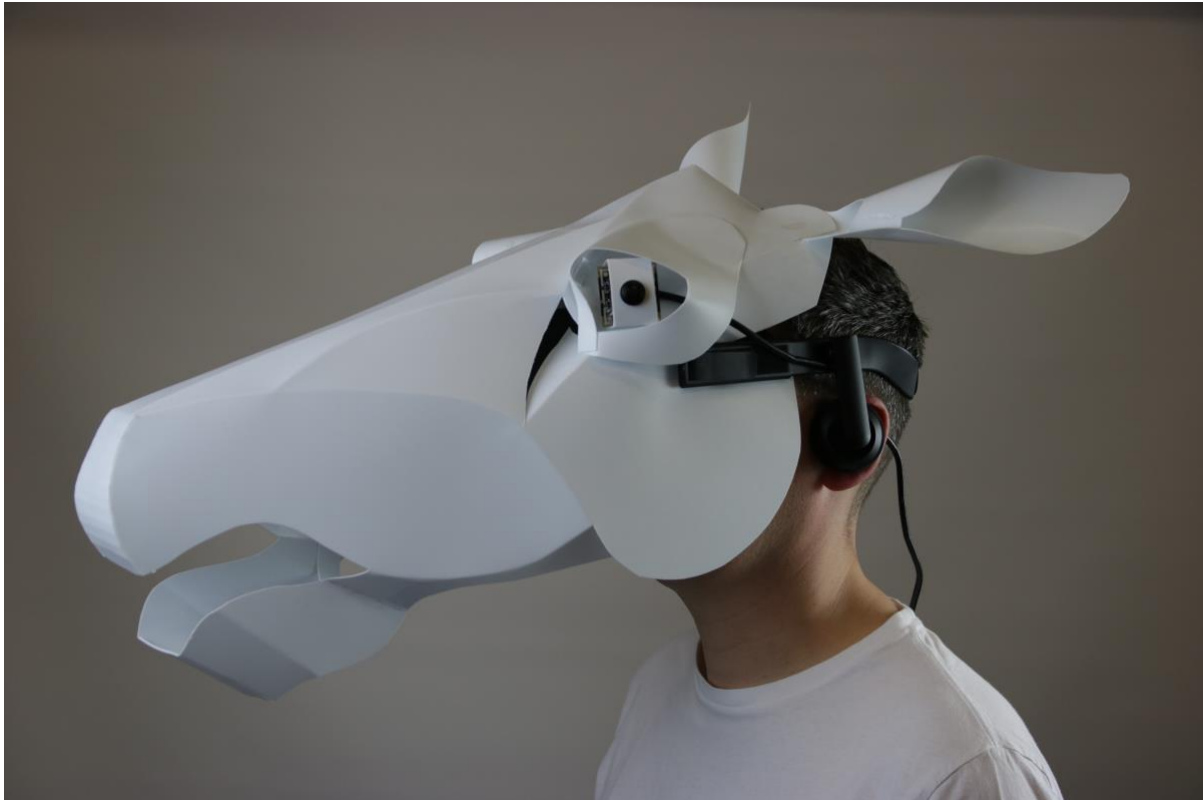
Figure 3: Prototype with 180-degree FoV cameras to create a 350-degree FoV with dichromatic colour range. Photo: Vincent O’Callaghan.
